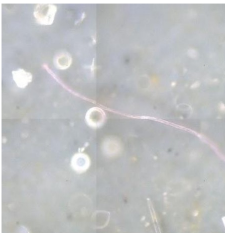
Images clockwise: The microRamen machine used for microplastics analysis, PhD student Laura Fantuzzi, examples of types of microplastics found in 2024: some spotted blue Teflon, a green paint fleck and a long pink PET fibre
